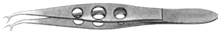
Rubman-Bores Corneal Fixation Forceps Curved. Overall length 103 mm, with 2 point fixation, tips separated by 3 mm 1x2 teeth each tip 0,12 mm PAB-384.10
